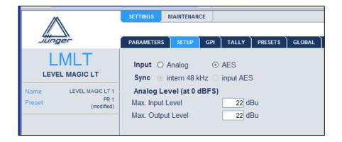
Here you can choose the used input. If AES is chosen, the Level Magic LT synchronizes to the digital input. If you use the analogue input you have to choose if you want to work with the internal SYNC 48 kHz or with an external taken from the AES input.
