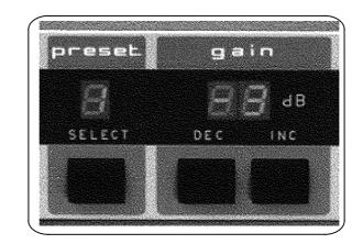
Press the PRESET button to select the one of the four operating programs of the unit which best corresponds to the kind of audio programme material which is being processed. Each operating program has optimum values of dynamic control characteristics (such as attack and release times etc.) for a different type of programme material.
