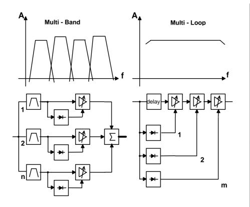
fig. 1: basic principles of dynamic range processors
