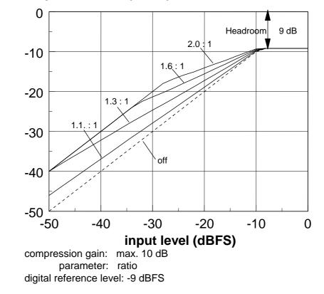
The audio signal delay through the dynamics processor is approx. 2ms due to delaying of the audio signal using internal memory. A small delay is deliberately introduced to the audio signal in order to allow limiter and compressor algorithms which can 'preview' the audio signal before changing it. That is the signal curve can be changed before maximum level is reached. (For further details see chapter 1).
