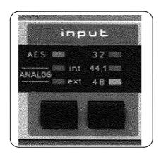
By pressing the left button in the input section the required input signal can be selected. Each time the button is pressed the input selection is changed and one of the three LED's above the button lights to show the newly selected input.
