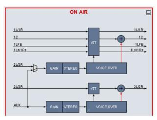
The program signal path for **program 1** is **5.1** while the **program 2** path is **stereo**.
