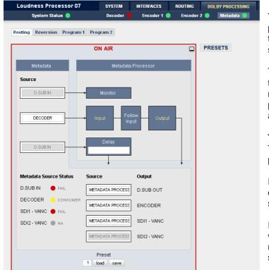
The metadata system of the **T**\***AP** has three paths. An independent monitor will allow for the evaluation of an independent metadata set, selected by its **Source** drop down box.
