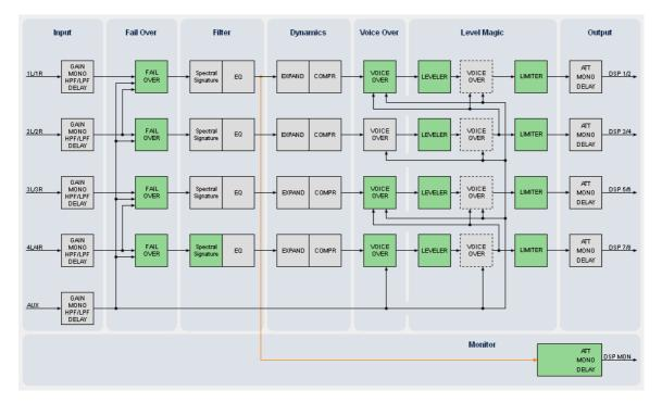
The processing blocks in use, which may be activated from their individual setup panes, will be indicated in green. Blocks shown in grey are not activated by the user. The location of blocks with dotted lines within the signal path depends on the block setup.
