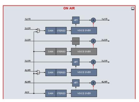
The program signal path (e.g. 1L/1R) includes an attenuator to reduce the program level and a node to mix the voice over signal with the respective program. As a source for the voice over signal you may select either the adjacent program input **2L/2R** or the **AUX** input. This allows you to build 2 fully independent voice over paths or up to 4 voice over paths with a common voice signal driven from AUX input.
