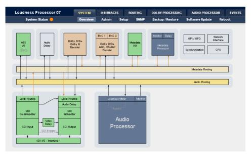
The graphical overview shows the main building blocks of the device including the options installed such as Dolby OEM modules or interface modules.
