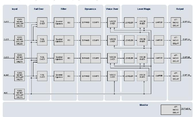
Audio processing block diagram 4 x 2 program configuration :
