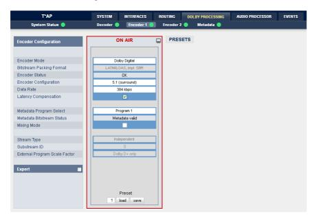
B) Two encoders mixed for Dolby Digital plus encoding and for AD (audio description) application :
