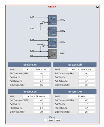
The source for the Fail Over circuit can be either the adjacent program input (e.g. input 2L/R for the program input 1L/1R) or the **AUX** input. The Mode switch will select the respective signal path.
