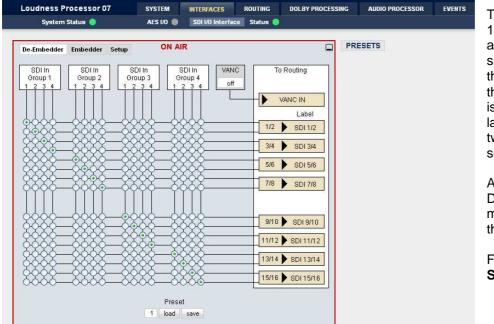
The **De-Embedder** has a 16 x 16 matrix to allow for any combination of audio signals to be presented to the **T\*AP** because inside the **T\*AP** the signal routing is oriented in pairs. I.e. the label "SDI 1/2" represents two audio channels selected by the matrix.
