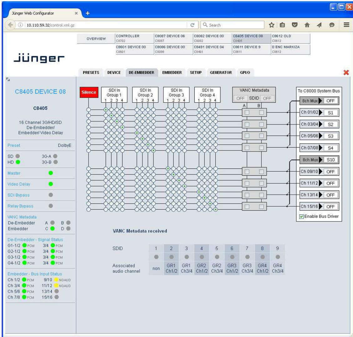
On the **DE-EMBEDDER** page you will get a matrix overview of the signals which are extracted from the SDI data stream and sent to the C8k audio frame bus. The de-embedder can route all of the 16 embedded audio channels in any combination to the C8k audio busses.
