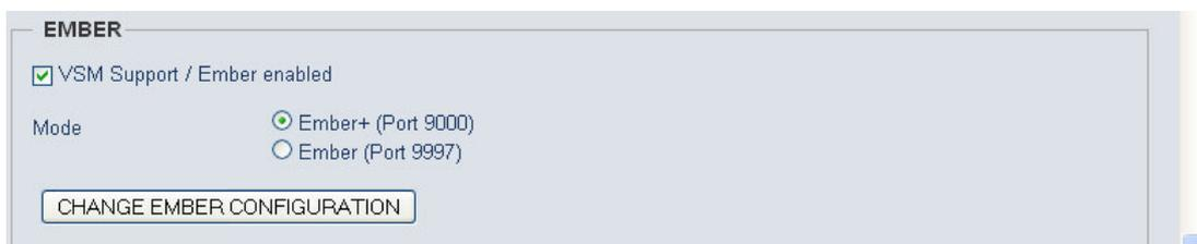
**VSM Support / Ember enabled** You may directly connect with a **VSM** application or use the Ember or Ember+ protocol to remote control the c8k frame.
