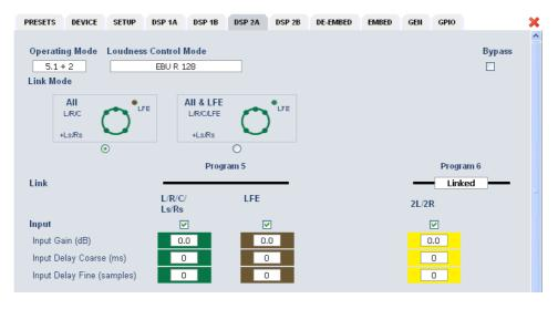
As mentioned above there is also a 5.1 + 2 program configuration available if you have bought the **surround option** for the C8492. In this case the first 6 channels of the DSP are linked for surround processing. This will also apply to **DSP 1** if 5.1 + 2 is selected. The example above shows a condition where the LFE is not linked to the other surround channels and may be controlled independently.
