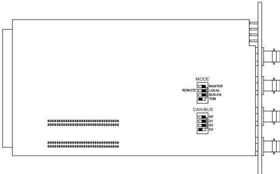
The **MODE** DIP-switch allows for setting of the operating modes:
