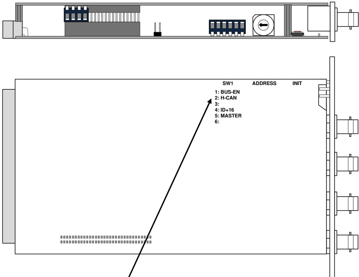
As a new feature you see the **CAN-H** switch above. That allows the module to operate with 1Mbit/s CAN-bus speed. This speed enhancement is helpful if you must log multiple programs from multiple **C8492s** in a compact 64 or compact 256 frame. Since only a selected number of modules will support the higher CAN-bus speed, grate care must be taken when setting up such a frame. All modules on the same CAN-bus must run on the same CAN-bus speed!
